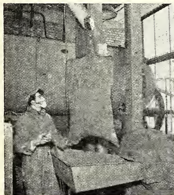
Left: A sack of bark is emptied on to a hopper from which it is fed into a disintegrator. Centre: The powdered bark is extracted with solvent. Right: The solvent is recovered for reuse. The plant, which is in accordance with Merz designs, was constructed by Rose, Downs & Thompson, Ltd., Hull.
